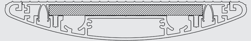
Treads — The treads are quiet underfoot, anti-slip, and the anodizing creates a hard, durable top surface. The treads can be up to 1200mm wide, and the large step depth (280mm) gives optimal walking comfort.
