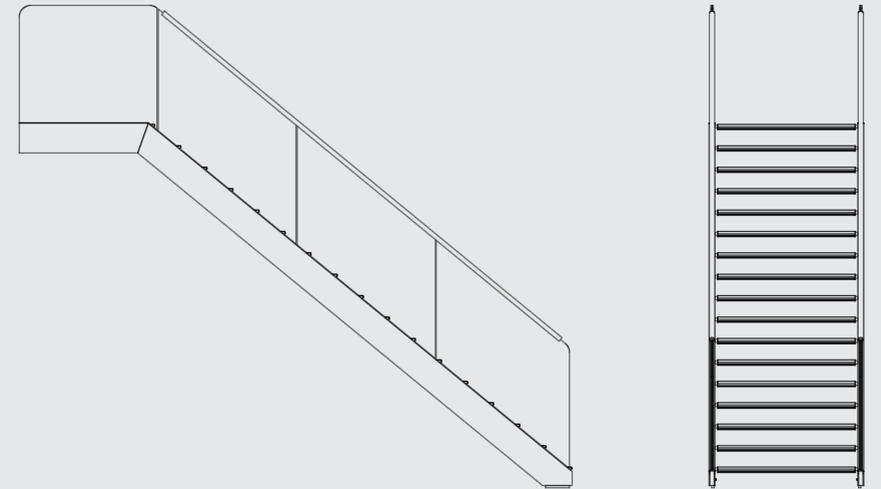
Stairs — The stairs have extremely clean lines, with crisp minimalist detailing. The stringers can be in any RAL colour. Handrails can be supplied in timber or stainless steel, and two types of glass for the balustrades. Another option concerns the stringers, which can be fitted with LED strips.
